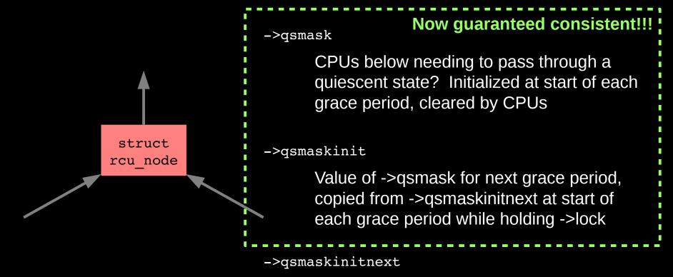
Value of ->qsmaskinit for next grace period, set and cleared by CPU hotplug while holding ->lock
