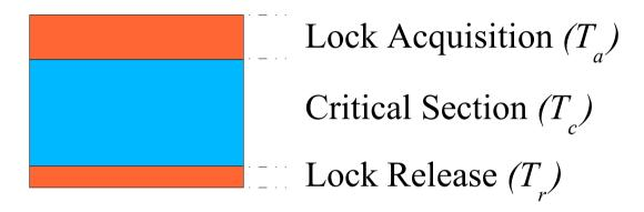
$$Efficiency = \frac{T_c}{T_c + T_a + T_r}$$
