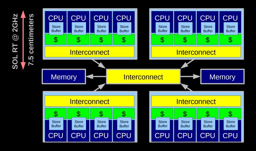
Electrons move at 0.03C to 0.3C in transistors and, so need locality of reference
